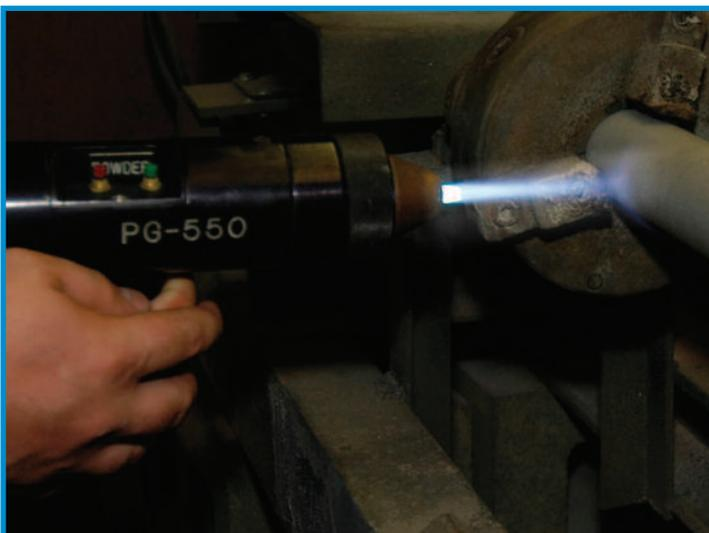
High Temperature Performance Coatings For Flame Spraying
